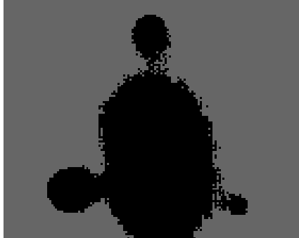
Fig. 9. Example of incorrect reconstruction of thermal conductivity at a depth of 2 mm caused by improper selection of excitation parameters.
